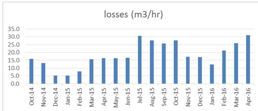
Figure 4. Month wise fresh water losses in m<sup>3</sup>/h
