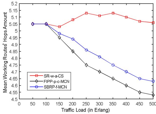
**Figure 3.** Mean working routes' hops amount versus traffic load considering the TID topology.
