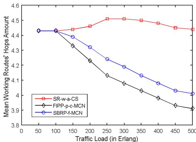
**Figure 7.** Mean working routes' hops amount versus traffic load considering the DT topology
