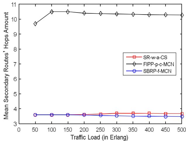
**Figure 8.** Mean secondary routes' hops amount versus traffic load considering the DT topology
