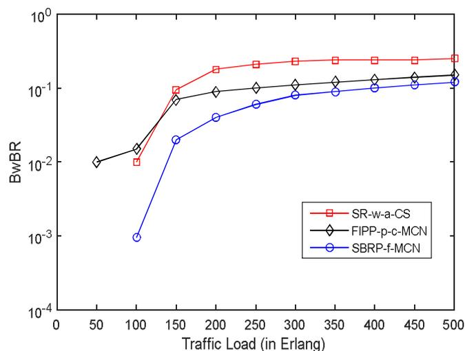
**Figure 2.** BwBP versus traffic load considering the TID topology
