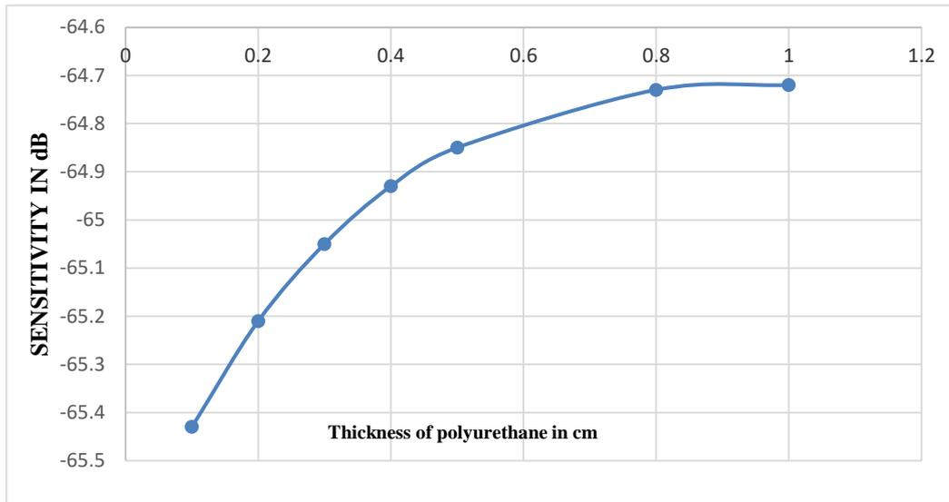
**Figure 6.** Thickness of Polyurethane versus Sensitivity
