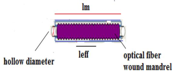
**Figure 2.** Direct view of the concentric Composite Mandrel
