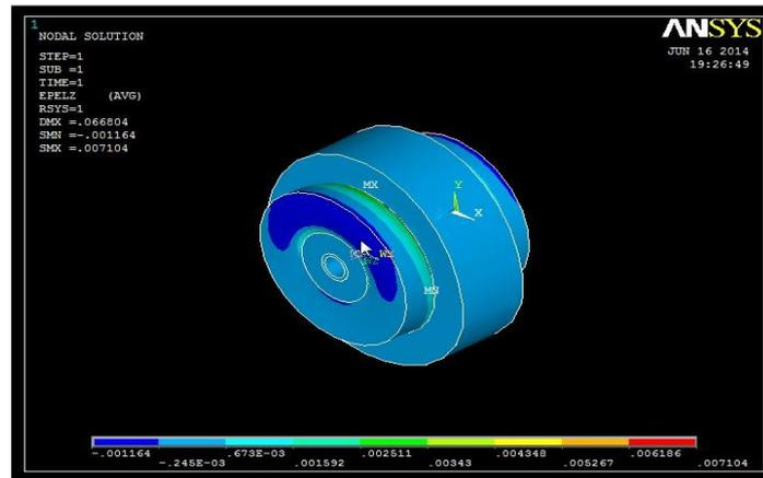
**Figure 5.** ANSYS Simulation of Axial Strain
