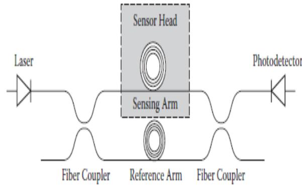
**Figure 1.** Mach-Zehnder Interferometer Principle
