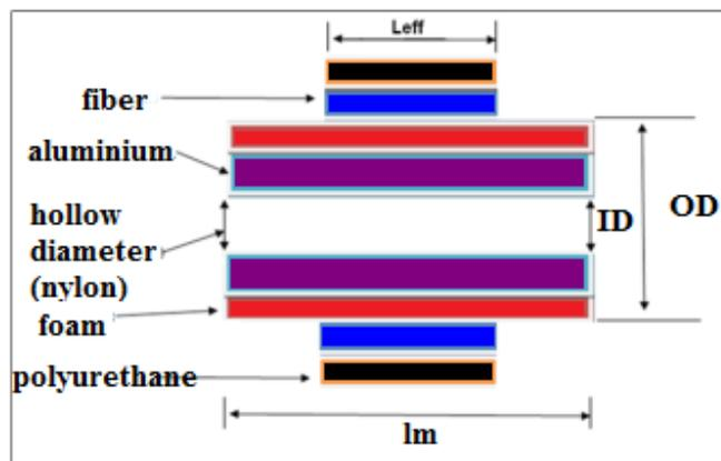
**Figure 3.** Cross sectional view of Novel MZI optical fiber wounded concentric composite mandrel
