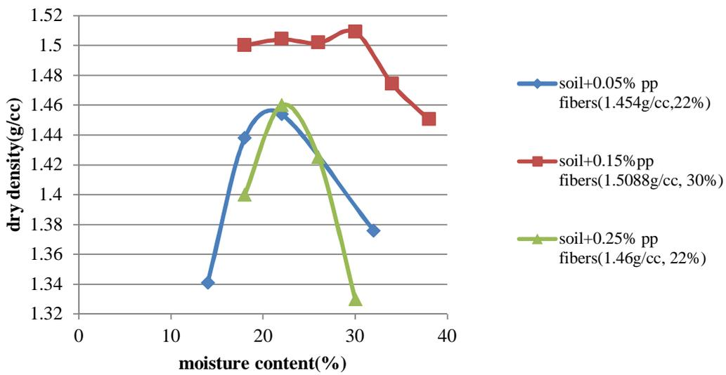
Figure 3. Results of black cotton soil treated with various percentages of polypropylene fibers
