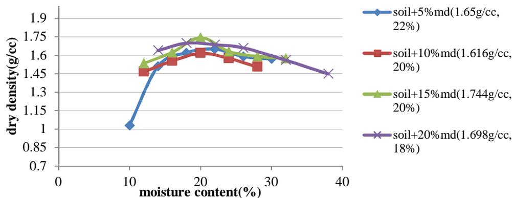
Figure 1. Compaction results of black cotton soil treated with various percentages of marble dust
