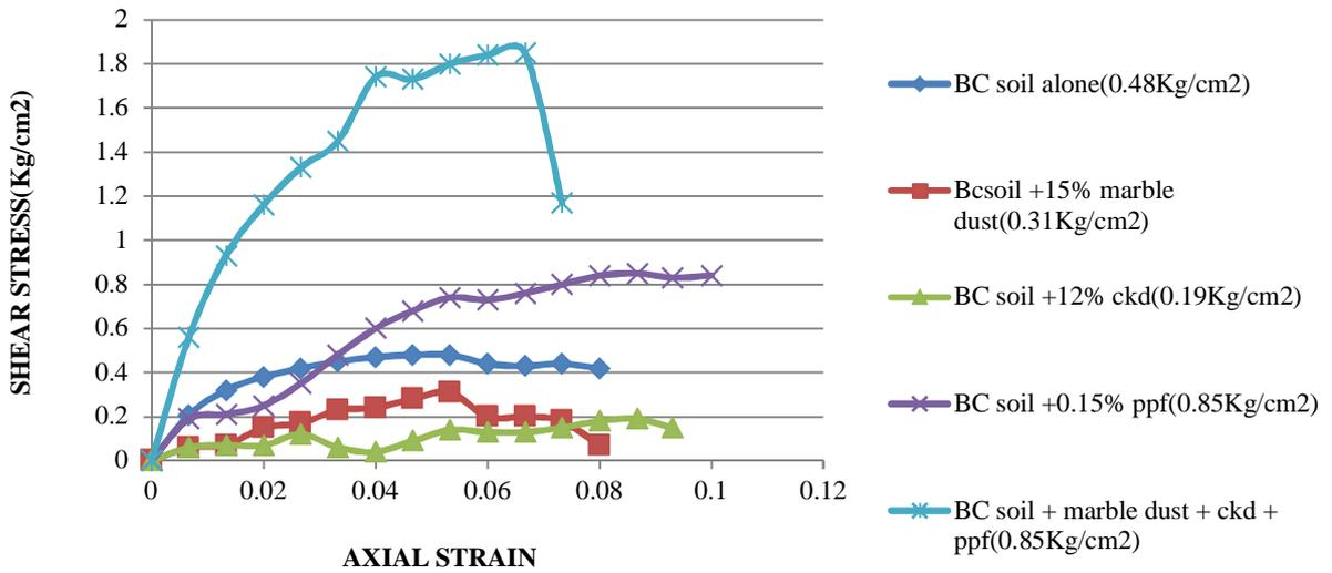
Figure 5. Comparison on UCC results between BC soil, BC soil with marble dust, cement kiln dust and polypropylene fibres and combinations of these admixtures immediately
