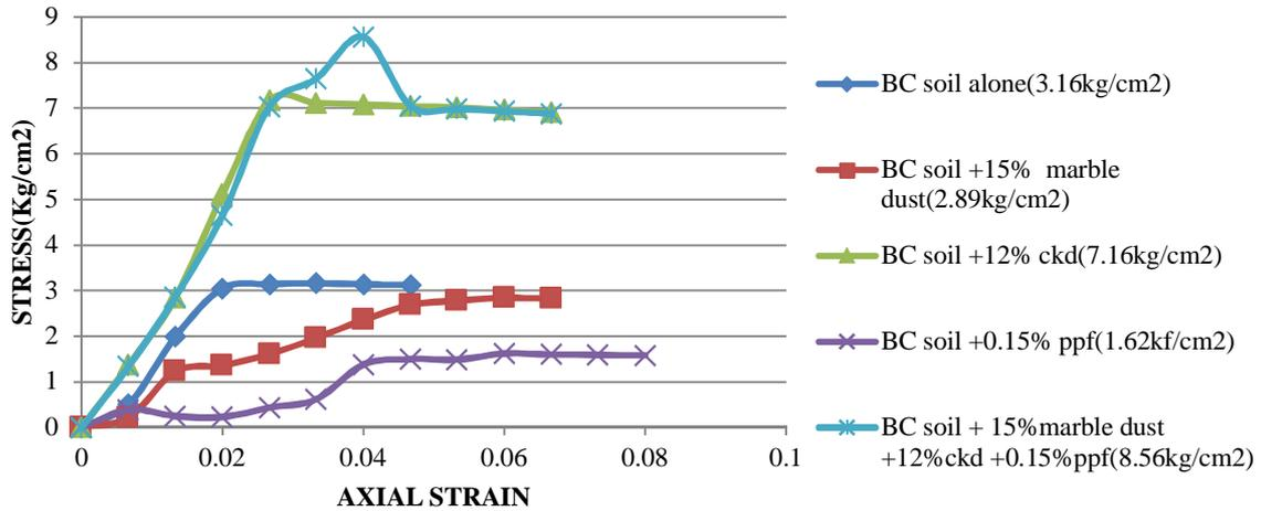
**Figure 7.** Comparison on UCC results between BC soil, BC soil with marble dust, cement kiln dust and polypropylene fibres and combinations of these admixtures at 14 days
