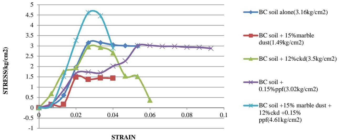
**Figure 8.** Comparison on UCC results between BC soil, BC soil with marble dust, cement kiln dust and polypropylene fibres and combinations of these admixtures at 21 days
