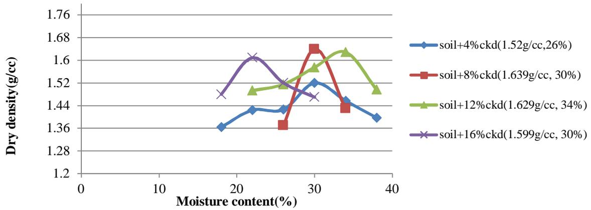
Figure 2. Results of Black Cotton Soil Treated With Various Percentages of Cement Kiln Dust
