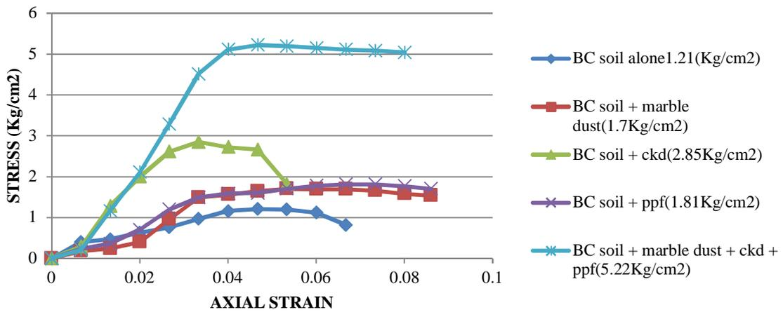
Figure 6. Comparison on UCC results between BC soil, BC soil with marble dust, cement kiln dust and polypropylene fibres and combinations of these admixtures at 7 days
