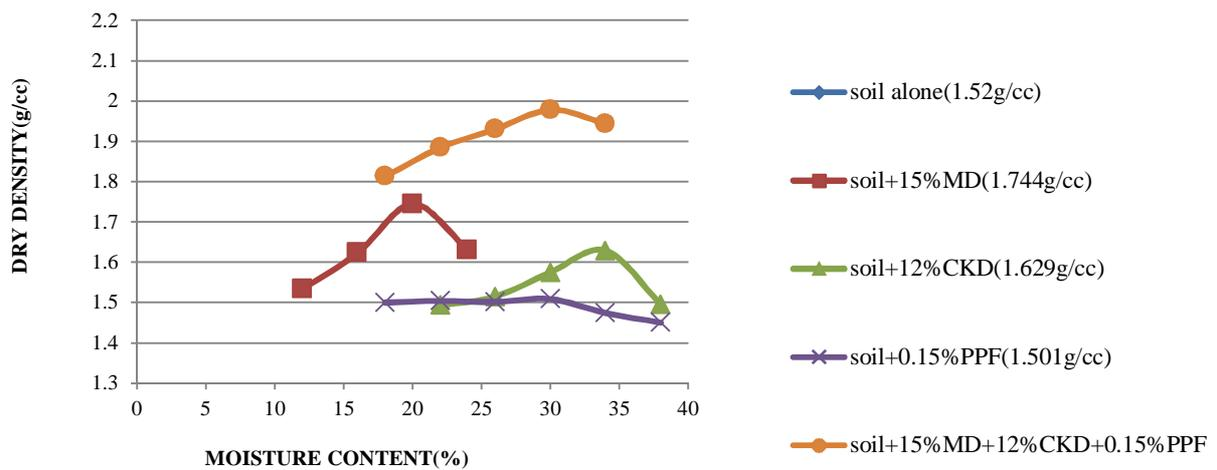
Figure 4. Results of black cotton soil and black cotton soil treated with optimum percentages of admixtures
